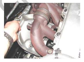
☐ Remove bottom exhaust manifold heat shield (3 - 8mm bolts).
