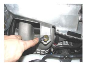
□ Remove intercooler – Loosen throttle body and turbo outlet hose clamps with either a flathead screwdriver or an 8mm wrench. Remove 3-12mm golden bolts holding the intercooler in place. Remove the intercooler while being careful not to damage the delicate fins. Stuff a couple rags in the throttle opening and turbo outlet to prevent small debris from entering while working.
