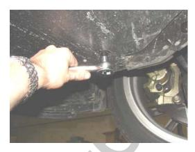
☐ Remove the plastic under pan (7-10mm bolts).
