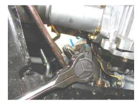
□ Remove two bolts in the gold colored pre-cat support bracket. If the engine is sagging and preventing clearance to these bolts, jack the engine up slightly until you can see the bolts. These bolts are best removed from a vantage point directly beneath them.
