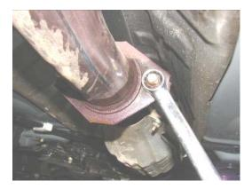
□ Remove the two 14mm bolts which are attached to the second cat. This will allow you to remove the center downpipe section and the cat.
