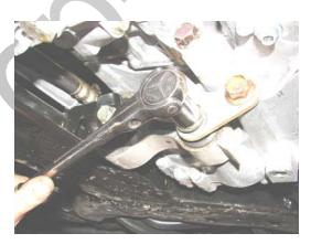
Remove the 17mm bolt on the small end of the wishbone engine mount. Loosen the rear bolt, but don't remove it. The engine will droop, but will still be supported by the top engine mounts. It isn't a bad idea to support the engine with a jack stand before removing the mount so the engine doesn't drop suddenly.
