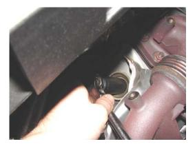
Remove the pre-cat oxygen sensor – Unbolt the two 10mm bolts retaining the O2 wires and set them out of the way. Now use a specific oxygen sensor socket to remove oxygen sensor. Use plenty of penetrating oil. If the sensor begins to drag **DO NOT FORCE IT.** You will damage the threads of the \$400 sensor. Work the sensor back and forth (alternate tightening and loosening) with lots of oil until it passes the tough spot and can be removed.
