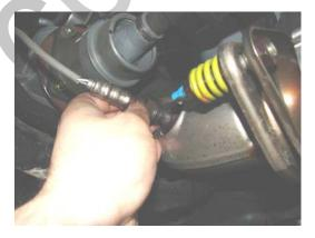
□ Spray rear O2 sensor with penetrating oil and remove it with an oxygen sensor socket.
