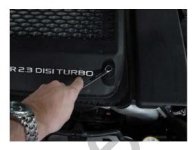
Remove the intercooler cover (2-10mm bolts). Unbolt the cover and pull it towards you to remove.
