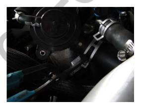
Remove the blow-off valve recirculation hose, and small vacuum line. Remove vacuum line to intake system. Use pliers to remove the torsion clip.
