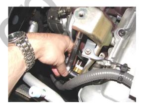
Remove the gold intercooler support bracket at the rear of the engine (2-13mm bolts).
