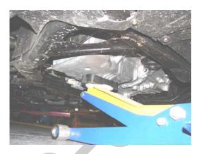
□ Support the engine with a jack under the oil pan.
