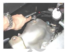
☐ Remove top exhaust manifold heat shield (5-8mm bolts).
