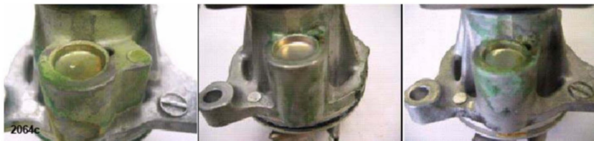
Water Pump NOT OK: Accumulation of crystallized coolant
