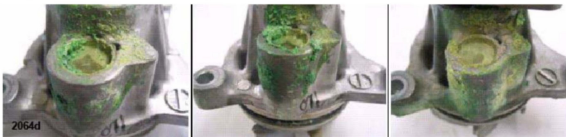
Water Pump NOT OK: Accumulation of crystallized coolant
